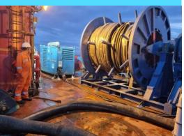
This spooler is driven via a Hanggluns motor and powered by our Deutz 913 diesel engine power pack.
